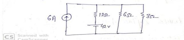
Q6. Find the Thevenin's equivalent circuit for the following diagram.
